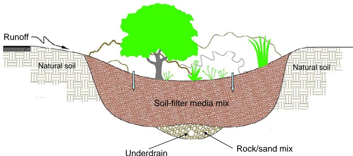
Figure 5-3. Modified Bio-retention System.
