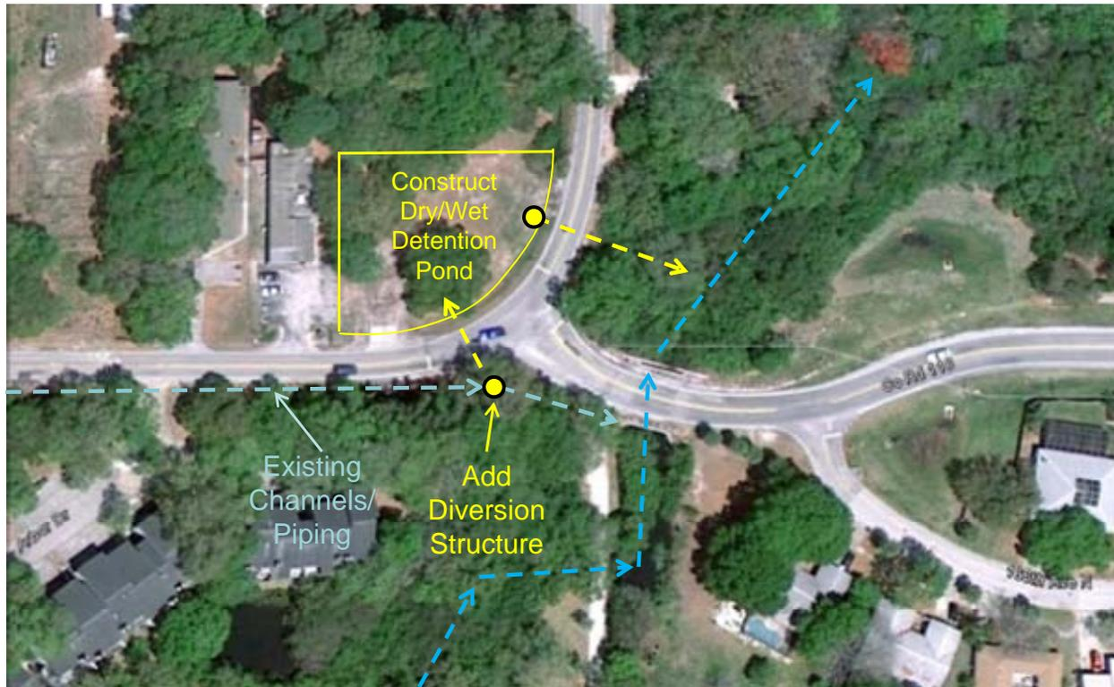
Figure 5-12. Alternative Conceptual Treatment System for the Whitney Road Drainage Swale.
